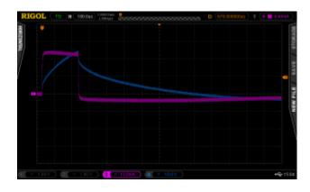
Resistance was read off the slope of the slanted IV segments in the XY timebase and capacitance was determined by I\*t/V in the YT timebase. The resulting circuit was assembled from an electrolytic
