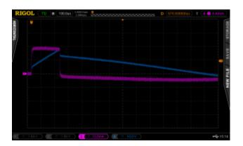
The model could be improved by adding a second resistor in parallel with the capacitor to obtain a proper sharkfin waveform rather than flat slopes, however I do not believe that it will be necessary to consider such a refinement for the purposes of designing an estim circuit. As it stands, distortions introduced by using different cheap capacitors (pictured below, 50V ceramic on the left and 50V electrolytic on the right) exceeded approximation error due to ignoring the parallel resistance.
