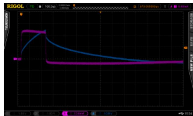
Resistance was read off the slope of the slanted IV segments in the XY timebase and capacitance was determined by  $I^2t/V$  in the YT timebase. The resulting circuit was assembled from an electrolytic
