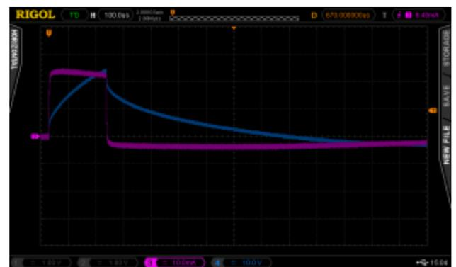
Resistance was read off the slope of the slanted IV segments in the XY timebase and capacitance was determined by  $I \cdot t / V$  in the YT timebase. The resulting circuit was assembled from an electrolytic
