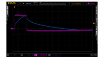
Resistance was read off the slope of the slanted IV segments in the XY timebase and capacitance was determined by I\*t/V in the YT timebase. The resulting circuit was assembled from an electrolytic
