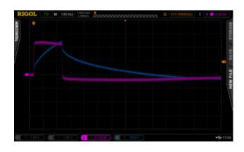
Resistance was read off the slope of the slanted IV segments in the XY timebase and capacitance was determined by I\*t/V in the YT timebase. The resulting circuit was assembled from an electrolytic
