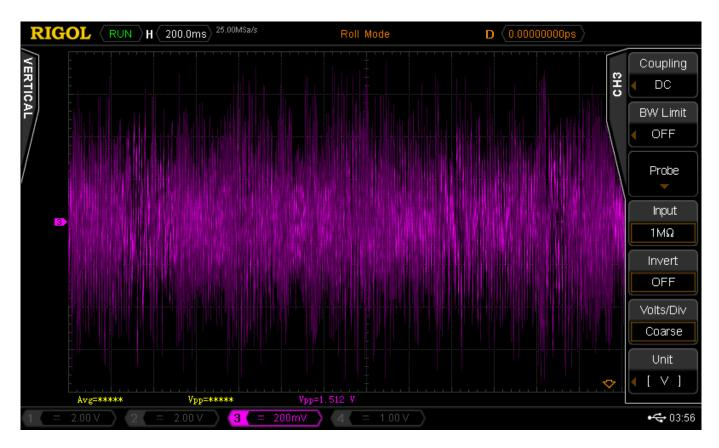
We can't drive an estim circuit directly from audio output – it can barely reach 1V at max volume let alone 100V+ – but can we use audio output to drive an off-the-shelf amplifier which in turn drives an estim? Here we measure the DROK TDA7297 12V amplifier. True to its name, it can boost ~1V audio to 12V:
