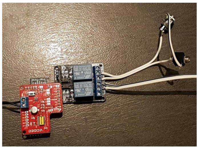
This picture is not for a USB relay but you get the idea... You will need to plug the USB into one side and each relay (blue in the above pic) will have 3 connectors (Com, NC & NO). A relay is like a switch that connects between Com and NC if no power sent to it and between Com and NO if power is on.
