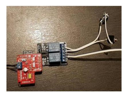
Ok so now needed to link every together to my equipment. I bought 2 3.5mm mono sockets and a 3.5mm patch lead. This allowed me to plug my e-stim butt plug etc direct to the relay and then use the patch lead to connect to my e-stim device without cutting any wires or messing with my expensive device. you will see from the picture the relay just switches the tip and the other contact is just passed direct from one socket to the other.
